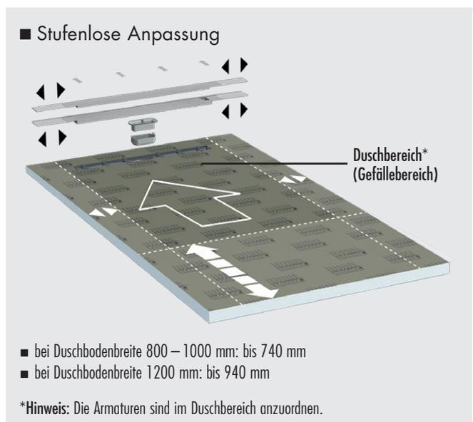
■ PRODUKTDATEN – LUX ELEMENTS®-TUB-LINE BOL V
