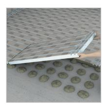
FLOOR-WH F ... is suitable for use on either wooden floors or mineral substrates such as concrete or screed. Using FLOOR-WH F 30 the fixing adhesive must always be applied over the full surface, FLOOR-WH F 50 can also be placed on dots (dots spacing  $\leq$  200 mm). For wooden floors, full coverage adhesion is always required.
