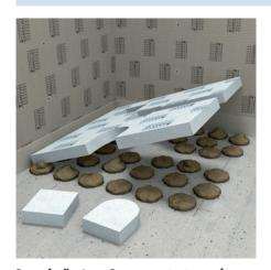
**Dots of adhesive** — For compensation in case of uneven substrates, to level the shower base element exactly horizontally. The spacing of the mortar dots should be approx. 20 cm, height compensation from 0- approx. 6 cm.
