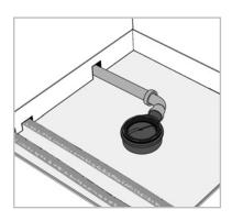
When installing a shower base, height compensation by means of TUB-U S 90 is useful above all when the TUB-U... substrate elements normally used in such cases cannot be installed e.g. when additional pipes run under the planned shower location or as height levelling for very uneven surfaces.
